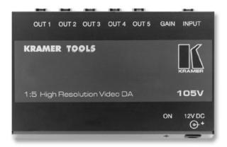
The Kramer 105V is a high performance distribution amplifier for composite video signals. It takes one input, provide correct buffering and isolation and distribute the signal to five identical outputs.
