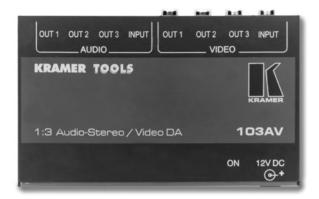
The Kramer 103AV is a compact distribution amplifier for composite video and unbalanced stereo audio signals. It will take one input, provide correct buffering and isolation and distribute the signal to three identical outputs.
