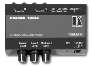
The **102MX** is a high performance 2 channel stereo audio mixer for line level and mic level audio signals. It mixes one line level input with either a microphone or a second line level input and produces a mixed audio output signal.
