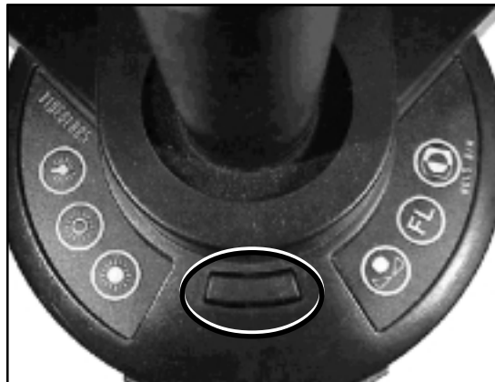
Figure 6 – The TeachCam's ON/OFF switch.
