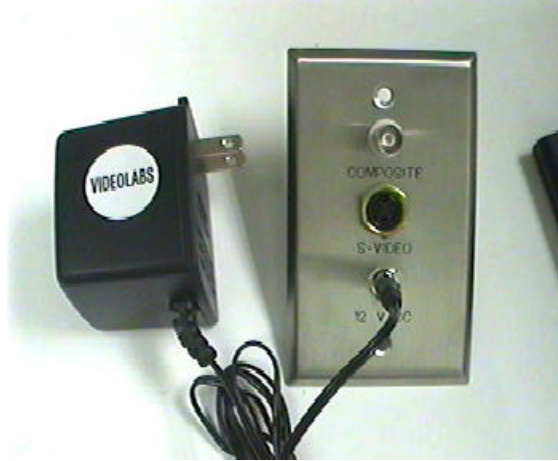
Figure 10: Power Supply Attached to Front of Wall Plate
