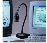
7890U Vision Viewer USB output with 640 \* 480 resolution, for high-quality digital imaging with simplicity and reliability.
