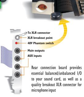
placed on the drive bay's front. There is an additional instrument input on the drive bay to allow those spontaneous instrument tracks in front of your computer. A stereo auxiliary input is provided so that your sound card's input can also be used for external devices when the MQ1 is switched off.
