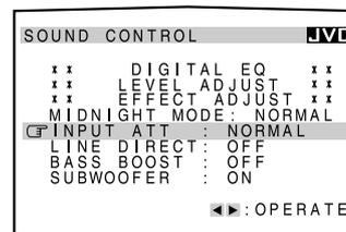
4. Press ◀ / ▶ to select the Input Attenuator mode “ATT ON” or “NORMAL.”
