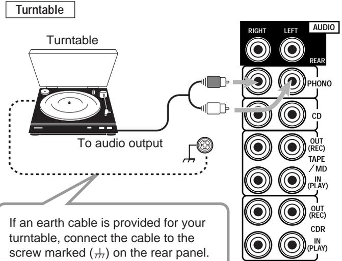
Ex.: This connection is for the turntable with an MM (moving-magnet) type cartridge.
