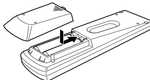
If the range or effectiveness of the remote control decreases, replace the batteries. Use two R6P(SUM-3)/AA(15F) type dry-cell batteries.
