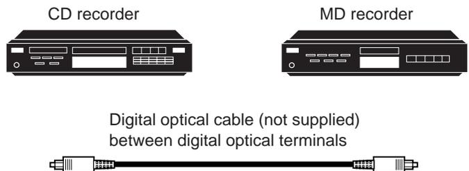
When the digital recording equipment such as an MD recorder and CD recorder has a digital optical input terminal, connecting it to the DIGITAL OUT terminal enables you to perform digital-to-digital recording.
