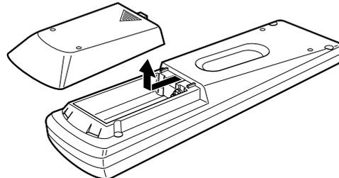
**2. Insert batteries. Make sure to match the polarity: (+) to (+) and (–) to (–).**
