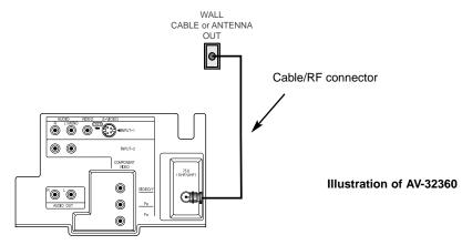
1) Connect an RF cable out from the wall outlet in to the RF Input on the back of the TV.
