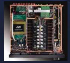
a thick ( $^{1}/_{16}$  inch), isolated base. This sophisticated design prevents digital and video noise from mixing with the delicate audio signals. Result: better sound quality.
