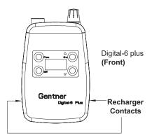
These contacts may be used in conjunction with Gentner's BC-10**B** for quick and easy recharging. Simply place the Digital-6 Plus receiver in the BC-10**B** charger. When not in use and it will automatically recharge for the next usage.
