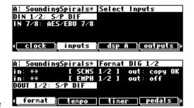
present at both the AES/EBU 1/2 output and the S/P DIF 1/2 output, but they can only be one *format*. S/P DIF selects a "consumer" format while AES/EBU selects a "professional" format. Use the AES/EBU format unless you have a compelling reason to do otherwise.
