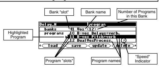
programs with a common theme are saved in a single bank. There can be as many as 100 bank "slots" in the internal memory of the DSP7000, and each bank contains 128 program "slots."
