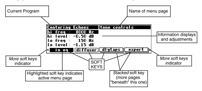
The upper left-hand corner of the display always shows the name of the program currently running. In the example shown above, we're running the program "Centering Echoes." The upper right-hand corner of the display always describes the menu page you're looking at. In the example shown above, we're looking at the "tone controls" menu page.
