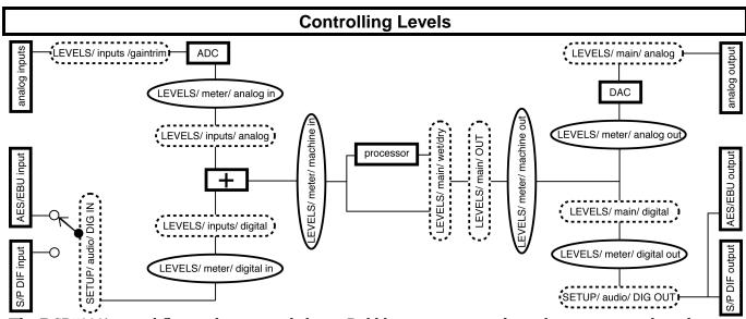
The DSP7000's signal flow is diagrammed above. Bold boxes represent physical structures inside and outside the DSP7000, for example, the analog inputs. Dashed boxes represent parameters that impact signal
