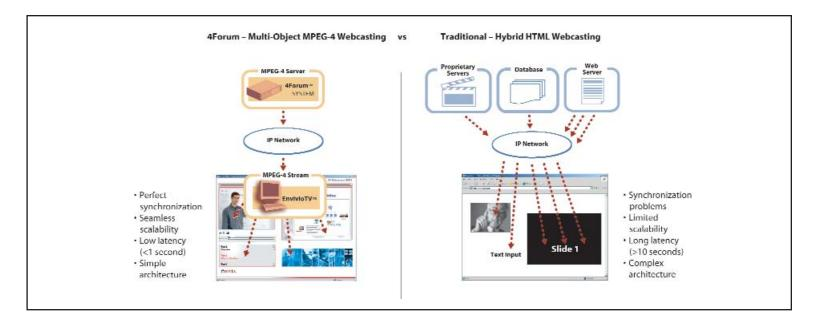
and collaborative material. It is an integrated plug-and-play and easy-to-operate system. The 4Forum appliance works on existing IP infrastructure, and content can be delivered over terrestrial, satellite, or wireless networks in multicast and unicast modes. Recipients can view the content on all major media players and on many devices, including PCs, TVs, and PDAs.
