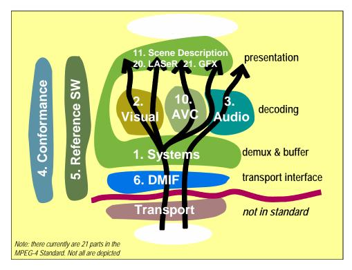
Figure 14. The parts of MPEG-4. The arrows represent the flow of bits through the MPEG-4 system.
