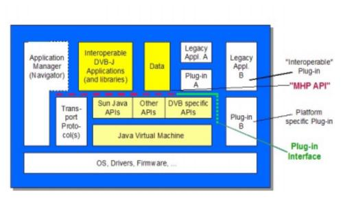
Figure 17. MHP reference architecture showing role of DVB-J
