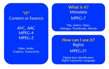
Figure 12. The Metadata and Rights Standards MPEG-7 and MPEG-21 are designed to complement coding standards MPEG-1, -2, and -4. Courtesy Streamcrest Associates.
