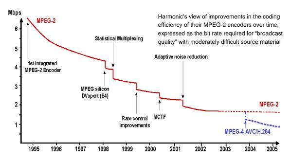
Figure 3. Improvements in coding efficiency are facilitated by MPEG-based competition. Courtesy Harmonic.
