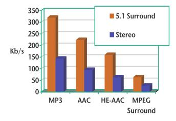
Figure 2. The evolution of MPEG Audio codecs has produced a 5 to1 reduction in bitrate for similar perceived quality.
