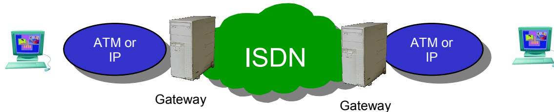
Figure 7. From H.323 (IP) to H.323 (IP) over ATM or ISDN
