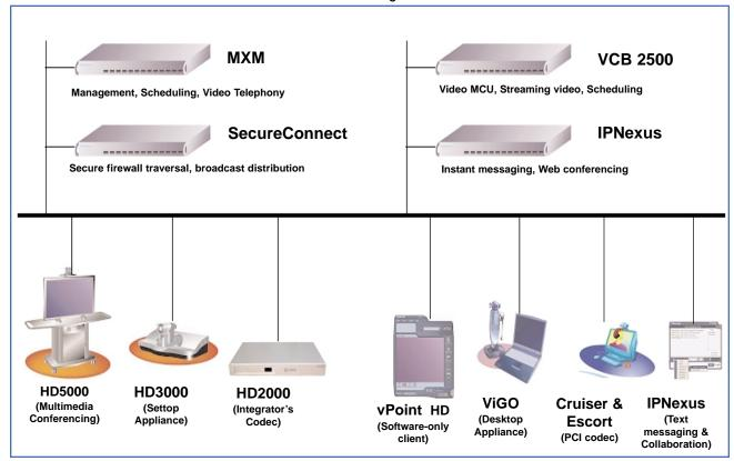
VCON's rich media conferencing solution is delivered via a client/server architecture, which dramatically decreases the total cost of ownership and allows unprecedented scalability and manageability. The desktop client applications are increasingly software-only. Such "thin" clients are easy to distribute, install, upgrade and maintain. The clients VCON offers are as follows:
