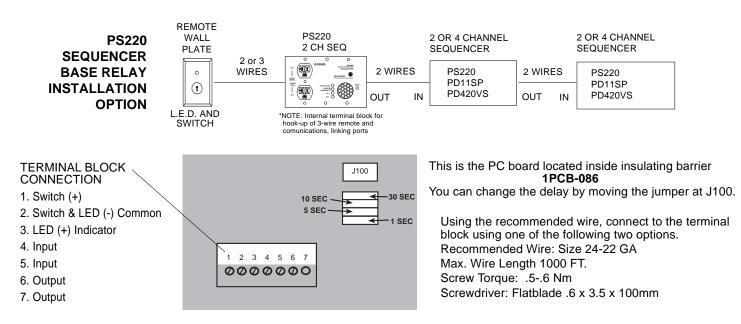
REMOTE LED INDICATOR: This can be used with remote switch as a remote unit activity indicator. A flashing LED indicates the unit is actively sequencing. When the LED is on constant the unit is completely "ON" or "OFF." To use this feature the (-) negative short lead of the LEDs is connected to terminal 2, and the (+) positive long lead of the LED is connected to terminal 3.
