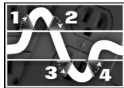
1. Voltage reaches an unsafe high level and the PD11VABP disconnects.
