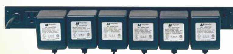
Back View PD9LV/L - Accommodates 6-7 AC adapters (wall warts)
