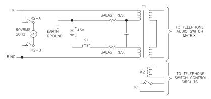
Figure 5. Subscriber-interface circuit
