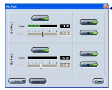
✓ Microphone volumes can be automatic (note here that Automatic Level Control is enabled). Acoustical Echo Cancellation and Noise Cancellation are also enabled. This screen, from the RAV 600, shows two microphone pods; the RAV 900 supports three microphone pods.
