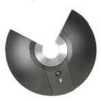
These are the microphones that are placed on the conference table. Two "pods" are included with the RAV 600, three with the RAV 900. Each pod contains three professional-grade microphone elements with automatic level control capability. Each pod's three elements work together to provide full 360° coverage. Multiple pods are daisy-chained from the mixer using standard Cat5 cables with RJ-45 connectors (included). Each pod features a
