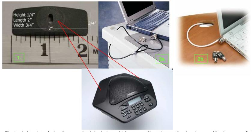
The basic idea is to fasten the security slot adapter, which comes with a strong adhesive, to one of the two upper flat surfaces on the MAX phone, and then connect any of the standard Kensington cable locking systems to that slot. Information on procuring the security slot adapter, along with two suggestions for cable locks is listed below:
