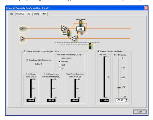
The AEC tab shows a signal flow diagram for AEC, and has the following features: **Enable AEC, PA Adapt and AEC Reference, NLP (Non-linear Processing), and PTT (Push-to-Talk) Mode**.
