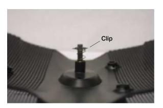
If the clip is placed too far away from the end of the rod, the spring will be more compressed which drives the rod into the switch on the PC board and prevents the button from recoiling (see Figure 2). When the button does not release properly, the mute will not turn on or off on the AccuMic II unit.
