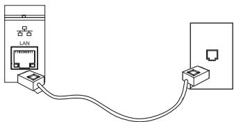
Figure 2.7. Connection to network
