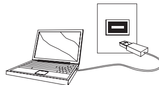
Figure 2.17. Connecting a computer through the USB
