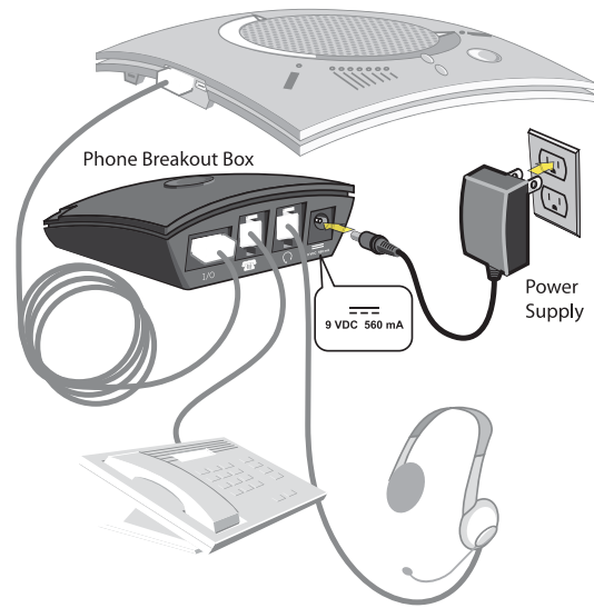
FIGURE 2.5 Connecting Chat 150 to a Telephone, Step 5
