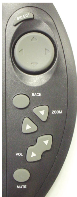
Figure 3.7 (E) Navigation, Zoom, and Audio control keys
