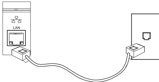
Figure 2.7. Connection to network
