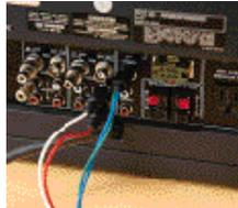
3. Connect the S-Video jack from the main cable to the video-in jack on your TV/VCR. If the TV/VCR is not S-Video capable, use the composite (RCA) video jack on the main cable.
