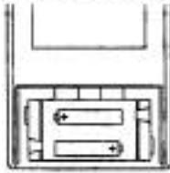
Insert two AAA (R03) batteries as indicated on the remote control unit.
