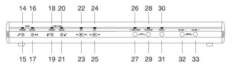
Figure 14. GT724 front panel controls
