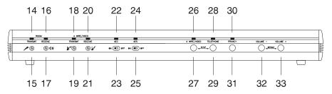
If using RS232 touch tones, it is not necessary to hit the TELEPHONE button [29]. When using the D serial-port command, the GT724 automatically activates the two-wire (telephone) mode. See Appendix D, RS232 Touch Tones, Page 24.
