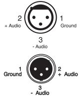
Figure 8. (Top) GT724 mixer audio female XLR connector; (Bottom) male XLR connector
