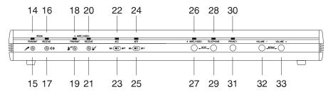
Under normal operating conditions, the ROOM TRANSMIT trim pot [15] is typically set at a 10 o'clock position or one-fourth open (Figure 17, left).
