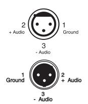
**Figure 12.** (Top) Four-wire (video) receive female XLR connector; (Bottom) four-wire (video) transmit male XLR connector
