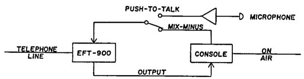
3. Cueing During the Broadcast. Normally you aren't able to cue the remote while they are on the air. This is because the cue audio is not totally rejected by the internal hybrid of the EFT-900 and therefore goes on air. For this reason, you must mute the receive audio during the cue period. If the cue is short, the short interruption in the program is hardly noticed by the
