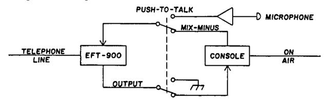
4. Using EFT-900 as a Telco Interface. When used with the ENCODE and DECODE switches in the OFF position, the EFT-900 can be used as standard telephone interface. You won't need to change your set-up either. The following diagram shows the basic set-up:
