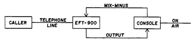
5. Using EFT-900 with TELEPROCESSOR. The EFT-900 significantly improves your telephone line quality. However, to maximize the sound of your phone line you can use the unit in conjunction with Gentner's TELEPROCESSOR, which adds equalization adjustments to your receive audio and maintains a consistent send level to your remote site. In addition, the TELEPROCESSOR has a built-in cue switch with condensor mic; this eliminates the need to build a separate cue circuit.
