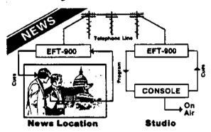
4. Call-ins. In addition to the above normal frequency extended applications, EFT-900 can also be used for call-ins. Since the product incorporates a preset internal hybrid your callers will be able to hear all the console audio for conducting normal conversations.
