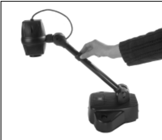
Figure 1 – Loosening and tightening the compression ring.
