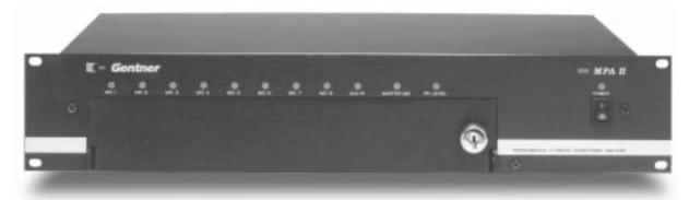
The MPAII is an eight channel, automatic gated microphone mixer and two channel power amplifier. The MPAII uses a microcomputer to control all mixing parameters, giving high precision and repeatability in performance. Additionally, installation and setup are easy with six pre-set programs for the most common applications. Six more programs may be configured by the user with a PC connected to the unit's RS-232 port. A locking front panel prevents unauthorized access to the controls.
