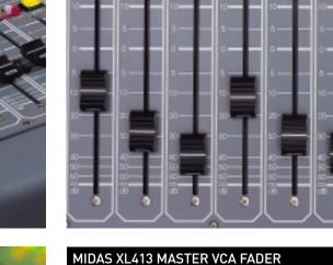
The XL413 Master Fader section provides moving fader control of the 10 VCA subgroups plus the two Grand Masters with solo and metering facilities. Isolate switches isolate the corresponding Group or Grand Master A/B VCA from the automation system. VCA Mute switches mute any post fade signal assigned to corresponding
