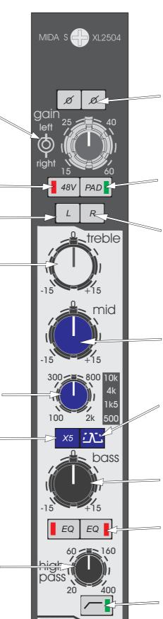
The PHASE switches activate a 180 degree phase change within the corresponding input amplifier.
