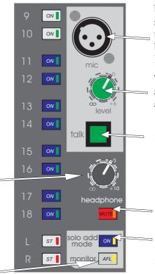
The TALK XLR socket accepts balanced 150 Ohm microphone signals from - 50dBu to - 20dBu and uses an auto ranging gain system to bring the level to nominal 0dBu line level.
