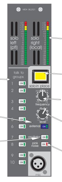
The METERS monitor the peak signal levels of the stereo AFL left and right solo busses or the PFL bus and local output level. The change over is automatic as part of the monitor AFL switch.
