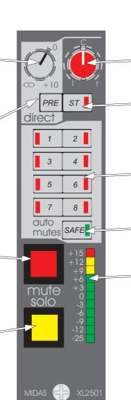
The PAN controls the placement of the channel within the master stereo mix and has a constant power law i.e. - 3dB at the centre position.
