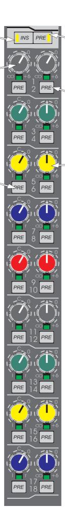
The insert PRE switch arranges the input channel signal to pass through the insert point before the equaliser when activated and after the insert point when not activated.
