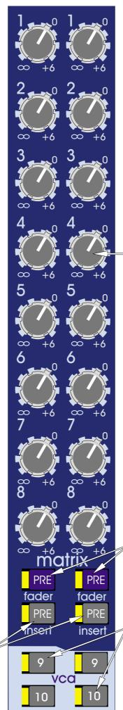
The matrix MIX controls (1 to 8) give continuous adjustment of the sub group levels sent to the matrix mixes from + 6dB to off.
