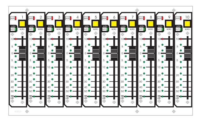
The vca MUTE switches act on any post fader input channels or audio sub groups which are assigned to be controlled from the corresponding VCA masters. The switches can be controlled from snapshot automation.
