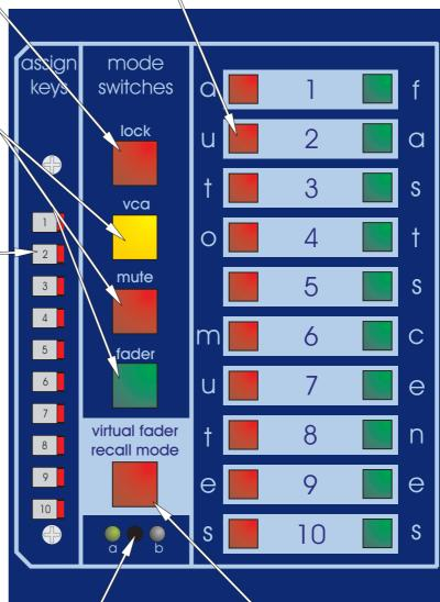
The VIRTUAL FADER key en/disables the operation of the virtual faders. It is only active if the console is unlocked to recall level.
