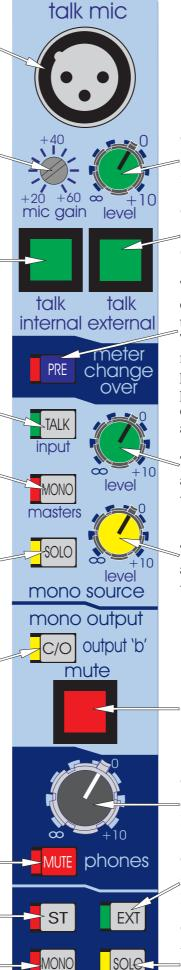
The talk LEVEL gives continuous adjustment of the post limiter signals from +10dB to off.
