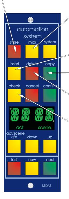
The MIDI key allows the operator to edit the snap shot MIDI information. On entering this mode the operator will be presented with a menu of the four MIDI messages that are stored within each snap shot, its operation is similar to the system menu.
