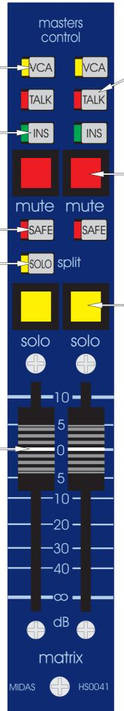
The TALK switches connect the matrix mixes to the MONITOR module. When the TALK INTERNAL or GENERATOR INTERNAL are active on the MONITOR module the oscillator, pink noise and talk mic can be routed into the matrix mixes.
