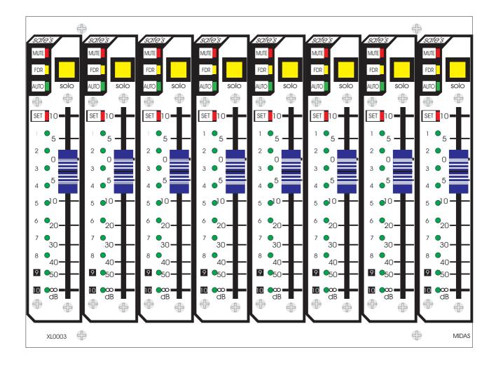
The SAFE switches disable remote control of the channels as follows:-
