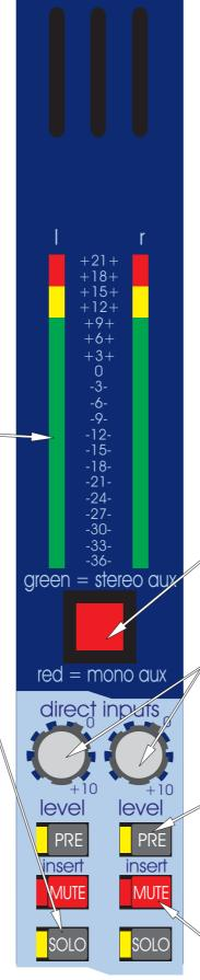
The global BUS MODE switches configure input module MIX controls to act as either mono aux (level and level), stereo aux (level and pan) or as audio sub groups (post fader and main pan). This makes the console extremely flexible and quick to reconfigure.
