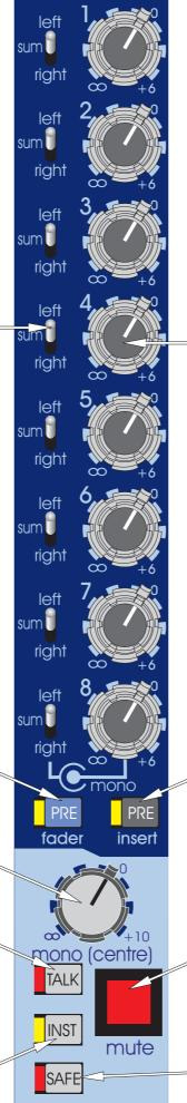
The matrix MIX controls (1 to 8) give continuous adjustment of the master levels sent to the matrix mixes from + 6dB to off. The top control adjusts the feed from the mono master and the lower control adjusts the feed from the stereo masters.
