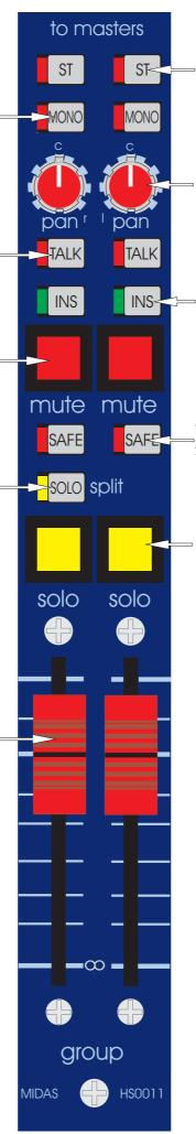
The ST switches connect the post fader sub group signals to the stereo master stereo busses via the pan controls.
