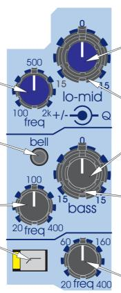
The LO MID (dual concentric top) control gives continuous adjustment of boost and cut from + 15dB to - 15dB with a 0dB centre detent.
