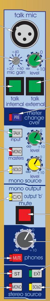
The talk LEVEL gives continuous adjustment of the post limiter signals from +10dB to off.
