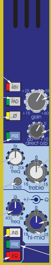
The GAIN control gives continuous adjustment of the input amplifier gain from + 15dB to + 60dB.
