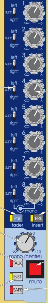
The TALK switches connect the stereo masters to the MONITOR module. When the TALK INTERNAL or GENERATOR INTERNAL are active on the MONITOR module the oscillator, pink noise and talk mic can be routed to the stereo masters.
