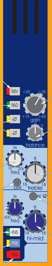
The GAIN control gives continuous adjustment of the input amplifier gains from + 15dB to + 60dB.
