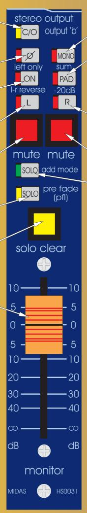
The MONO sum switch adds the left and right monitor signals with a 4.5dB summing loss.
