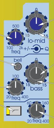
The LO MID (dual concentric top) control gives continuous adjustment of boost and cut from + 15dB to - 15dB with a 0dB centre detent.
