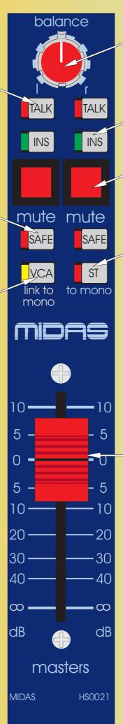
The BALANCE (pan) control gives continuous and reciprocal adjustment of the stereo left and right signal levels by + 3dB to off. This allows fine adjustment of the left, right power levels and imaging.
