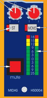
The MONO switch connects the post fader channel signals to the mono master bus.
