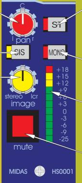
The MONO switch connects the post fader channel signal to the mono master bus.
