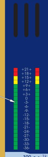
The METERS monitor the peak signal levels of the stereo left and right monitor paths.
