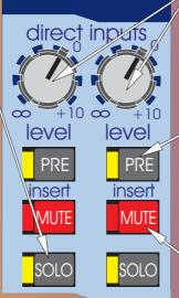
The DIRECT input controls give continuous adjustment of the direct input levels from + 10dB to off. The direct signals are summed into the sub group signals and can be used as effects returns etc. or for console bus linking.
