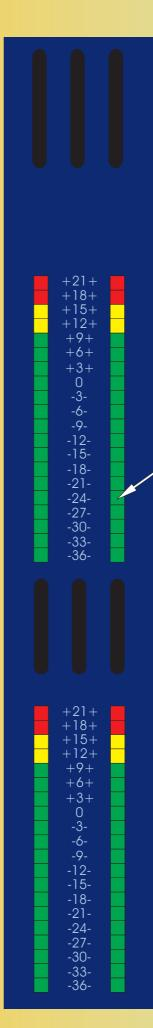
The METERS monitor the peak signal levels of the aux outputs (post fader).
