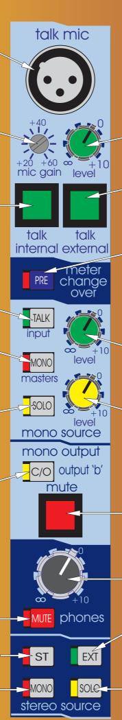
The talk LEVEL gives continuous adjustment of the post limiter signals from +10dB to off.
