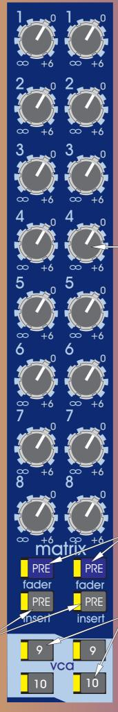
The matrix MIX controls (1 to 8) give continuous adjustment of the sub group levels sent to the matrix mixes from + 6dB to off.
