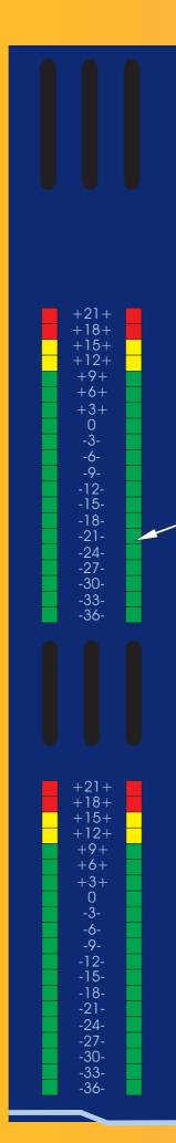
The METERS monitor the peak signal levels of the matrix outputs (post fader).
