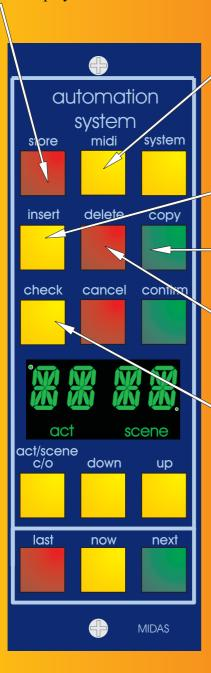
The COPY, DELETE and INSERT keys allow the operator to edit the snap shot sequence in the following manner.
