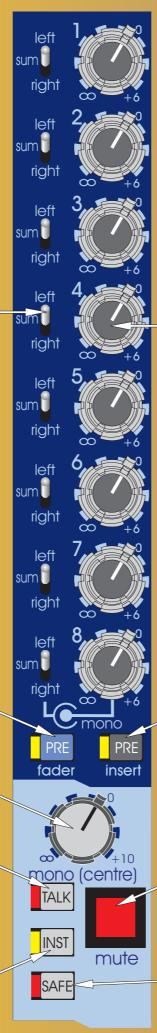
The TALK switches connect the stereo masters to the MONITOR module. When the TALK INTERNAL or GENERATOR INTERNAL are active on the MONITOR module the oscillator, pink noise and talk mic can be routed to the stereo masters.
