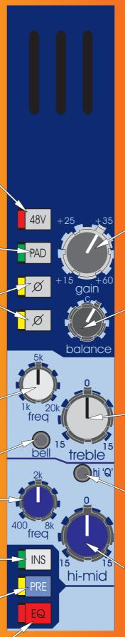
The GAIN control gives continuous adjustment of the input amplifier gains from + 15 dB to + 60 dB.
