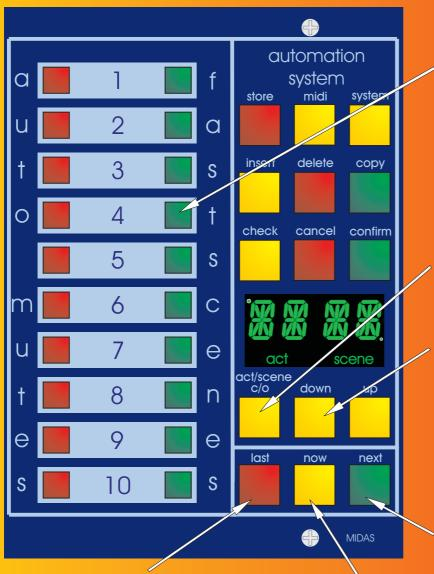
The FAST SCENE keys provide the operator with ten quick entry points into the ACT/SCENE sequence. I.e. if FAST SCENE key one is associated with ACT.SCENE 10.02, pressing it will recall ACT.SCENE 10.02.
