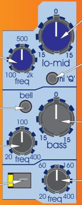
The LO MID control gives continuous adjustment of left and right boost and cut from +15dB to -15dB with a 0dB centre detent.
