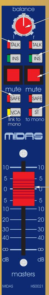
The BALANCE (pan) control gives continuous and reciprocal adjustment of the stereo left and right signal levels by + 3dB to off. This allows fine adjustment of the left, right power levels and imaging.
