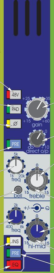
The GAIN control gives continuous adjustment of the input amplifier gain from + 15dB to + 60dB.
