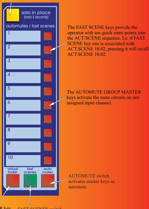
The VIRTUAL FADER key en/disables the operation of the virtual faders. It is only active if the console is unlocked to recall level.
