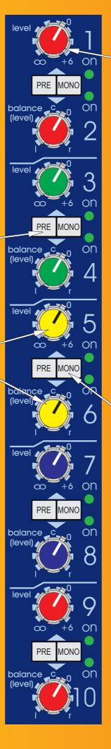
The 10 Aux send pots have individual ON/OFF switching using the consoles assignment system. A LED next to the function shows the Aux status. These assignments may also be stored as part of the Scene snapshot. By using a Matrix module and assignment system, various send levels can be achieved out to an effects unit during the show from each input module.
