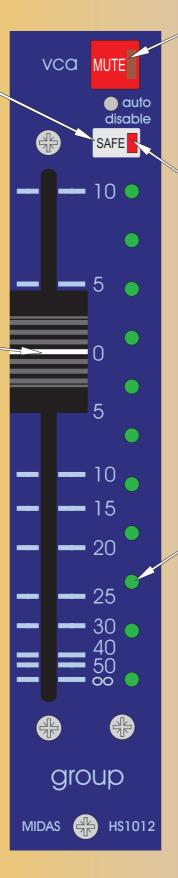
The VCA MUTE switch Mutes any channel that has been assigned to that VCA master. This mute can be stored as part of the console snapshot for scene recall.
