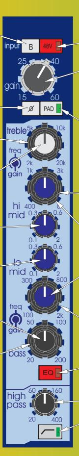
The 48V switch connects 48 volt phantom power to the input connector which is suitable for a condenser microphone or DI box.
