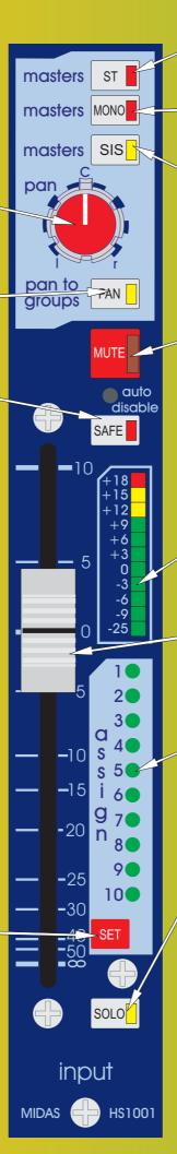
The ST switch connects the post pan signal to the Left and Right busses.
