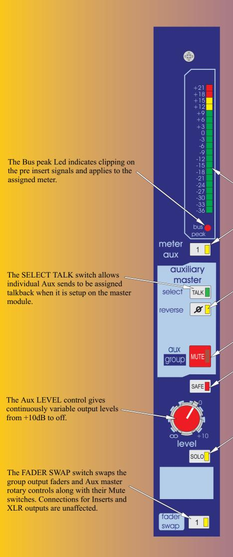
The METERS monitor the peak signal levels of the sub group outputs (post fader) or the Aux outputs (post Master level) depending on the METER TO AUX switch position
