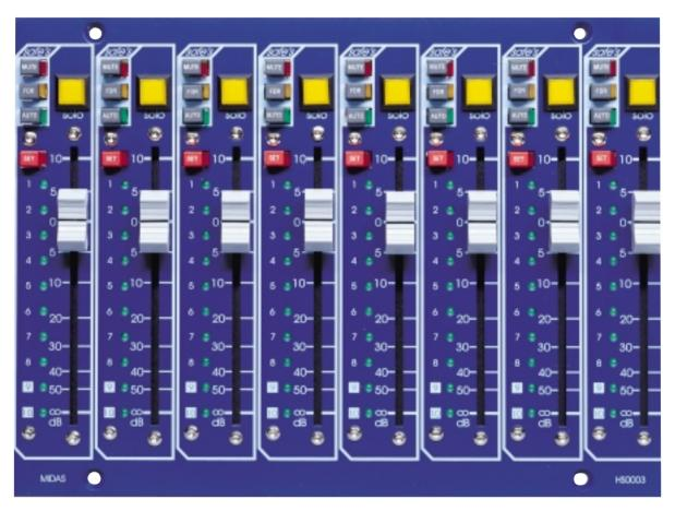
The Input faders of the HS0003 are linked to an intuitive, VCA level automation system, which is mainly controlled from the centre section of the console, though key status buttons and indicators are located adjacent to each fader. Each fader has a Automation Safe button that removes it from automation control as well as a Fader Safe button which removes the fader from any form of remote control.
