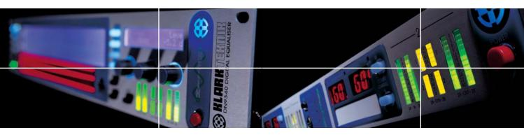
The DN9340 is a 2RU, dual channel device that condenses all commonly-used EQ functions into one unit, and adds a couple of new ones that are unique to Klark Teknik.
