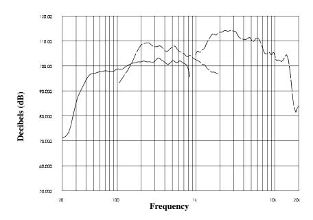
Figure 4—Variplex<sup>TM</sup> Typical Frequency Response with DX34A Digital Speaker System Processor Presets (swept sine-wave input, under anechoic environment; normalized response, from 4 volts at 500 Hz at 10 ft., with the microphone axis coincident with the aiming point, midway between mid- and high-frequency horn).
