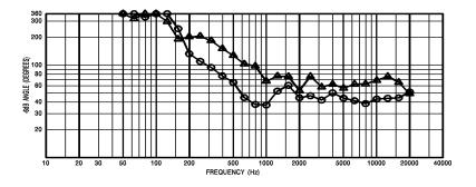
Figure 4—T252+ Directivity vs. Frequency, Whole Space (anechoic)
