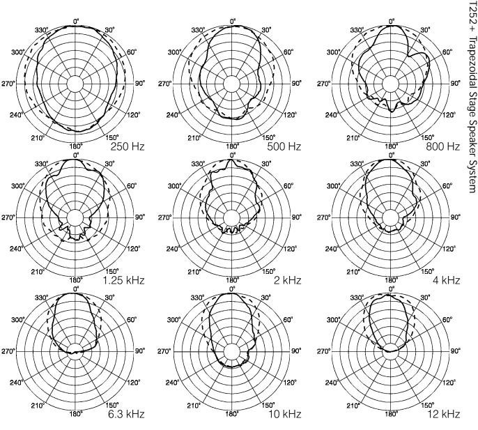
Figure 3—T252+ Beamwidth vs. Frequency, Whole Space (anechoic)
