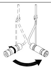
TWIST THE HOUSING OF THE MICROPHONE CLOCKWISE OR COUNTER-CLOCKWISE TO ROTATE THE POSITION OF THE MICROPHONE.
