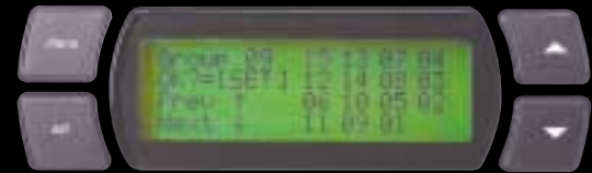
PRESSING THE SET KEY ACCEPTS THE GROUP, RUNS CLEARSCAN GROUP AND DISPLAYS THE OPEN CHANNELS IN ORDER OF CLEARNESS.
