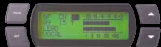
PRESSING THE SET KEY ACCEPTS THE CHANNEL, INSTALLS THE GROUP AND CHANNEL AND RETURNS TO THE MAIN SCREEN.
