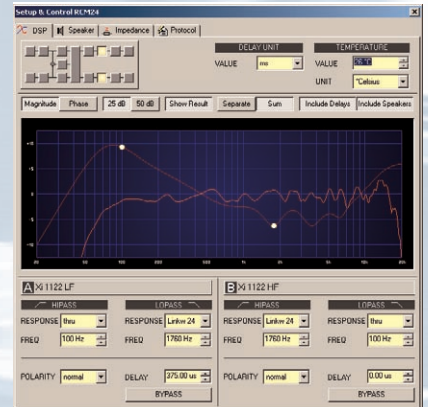
Crossover with each Hi and Lo-Pass per channel. Impact of all DSP parameters (filters, delay, level) to acoustical delivery of the system can be displayed.
