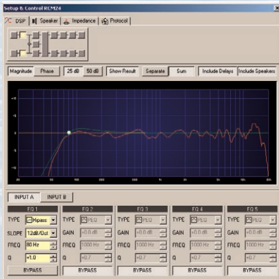
Channel-EQ with five filters. Display of the filters and their acoustical impact on the loudspeaker system.
