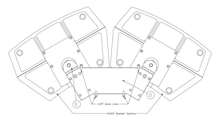
Figure 3A—Top/Bottom View of Frame Structure of a Three-Speaker Horizontal Array using Mb600 and Mb500 Brackets
