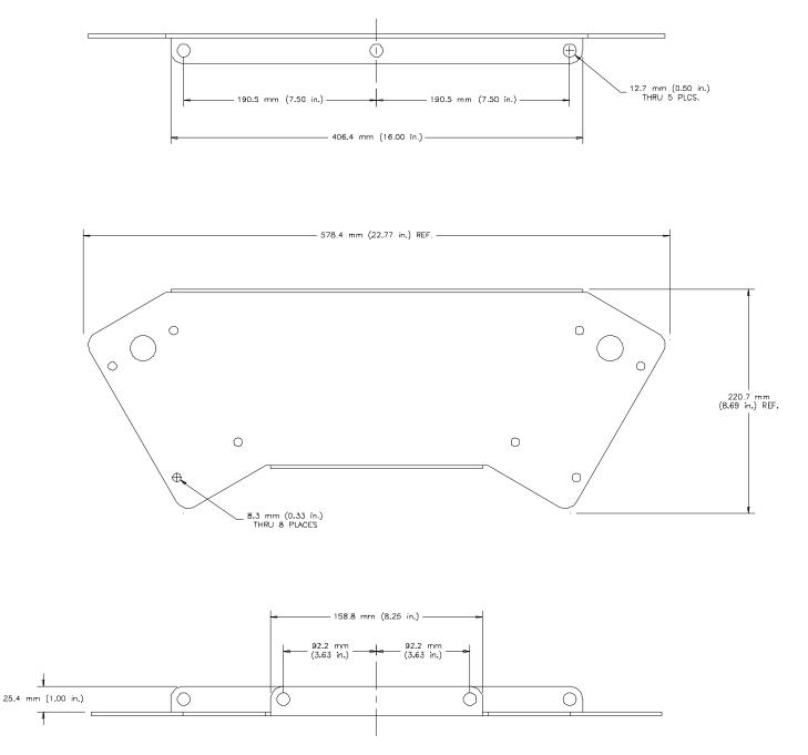
Figure 2—Top/Bottom View of Frame Structure of a Two-Speaker Horizontal Array using Mb600 and Mb500 Brackets
